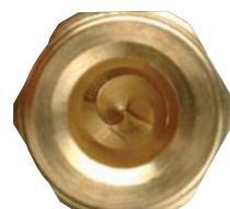
The picture shows the inside of a spiral nozzle with a completely free passage, without any internal vane.
