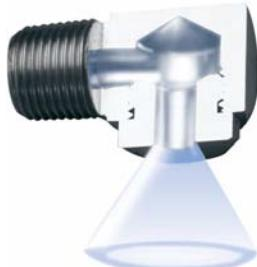
A hollow cone spray pattern consists of droplets concentrated onto the outer surface of a conical shape volume of water, with no droplets on the inside of the spray pattern. These nozzles are normally used for pollution abatement and gas cooling applications in addition to many other industrial processes.
